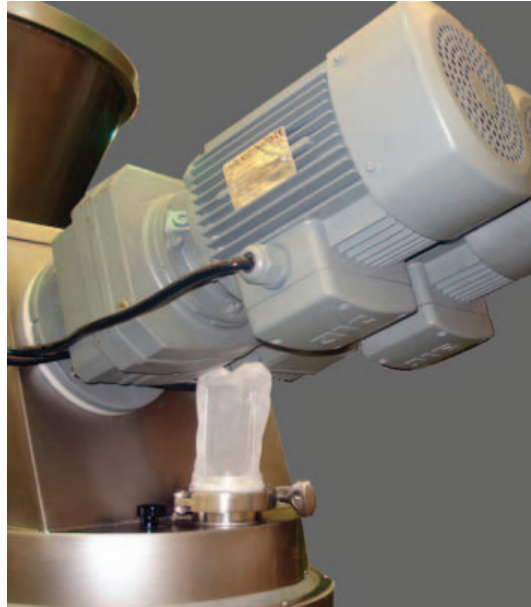
Double auger filling method (coarse and fine feed)
